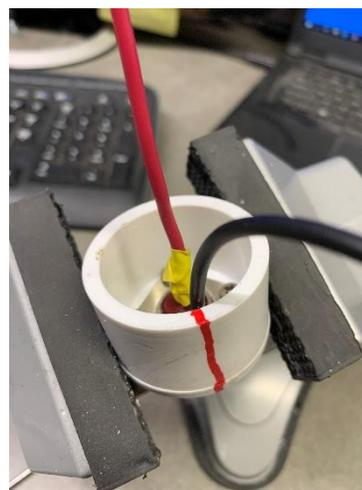
Mark in some way either side of the hub corresponding with one of the wires.
