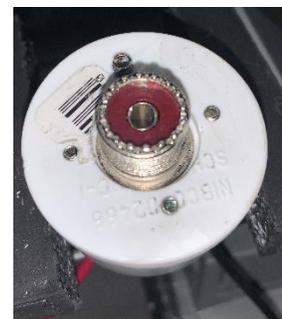
On the other side of the SO-239 two wires are connected which will be used to connect to each of the quarter wave wires.
