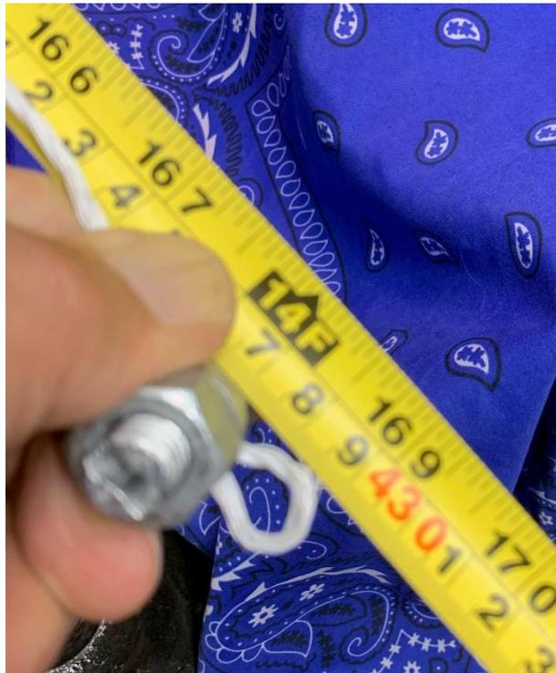
Each dipole element wire was carefully measured to see that its length matched what was earlier solved for. Note that while we were looking for 430 cm the picture shows only 329 cm. The other end of the element also had a lug as this end which was not included in this measurement. This accounted for an additional 2 cm so the total actual length here was 431 cm.
