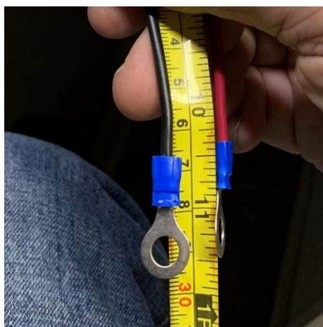
Try to keep the gap wires of the same length. While there is no electrical advantage, it will help avoid confusion in your calculations later.
