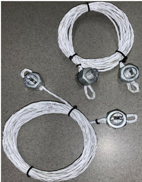
Shown above are the two dipole elements fully assembled and precisely cut to length. SPECIAL NOTE: Do not overtighten these lugs. Tighten them down finger tight and then an additional half-turn with a wrench. These things are mere cast iron and will easily rupture with too much torque.
