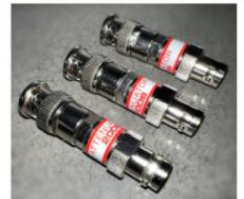
Three 20dB attenuators.
